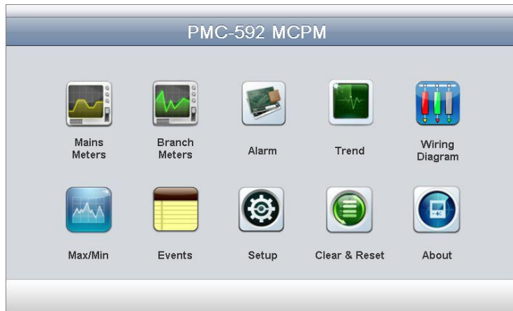
Figure 3-40 HMI's Main Display
